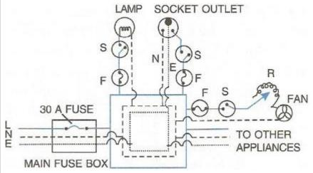
These appliances are connected to the mains in a parallel arrangement.
