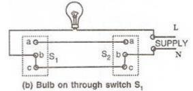
Similarly, on operating the switch  $S_2$ , the connection 'bc' changes to 'ba', which again completes the circuit [Fig. (c)].
